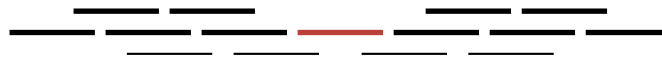
■ Figure 1 A unit interval graph where the subset of thick intervals is a maximum 2-IS with one isolated vertex. Note that exchanging the top four intervals with the bottom four intervals yields a maximum 2-IS with two isolated vertices, namely the first and last vertex.
